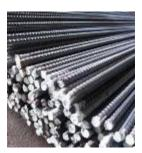
• Long products: Finished long steel products are normally produced by hot rolling/forging of bloom/ billets/ pencil ingots into useable shape/ sizes. These are normally supplied in straight length/cut length except wire rods, which are supplied in irregularly wound coils. The different types of long products include bar and rods, CTD/TMT, wire rod, angles, shapes and sections.
