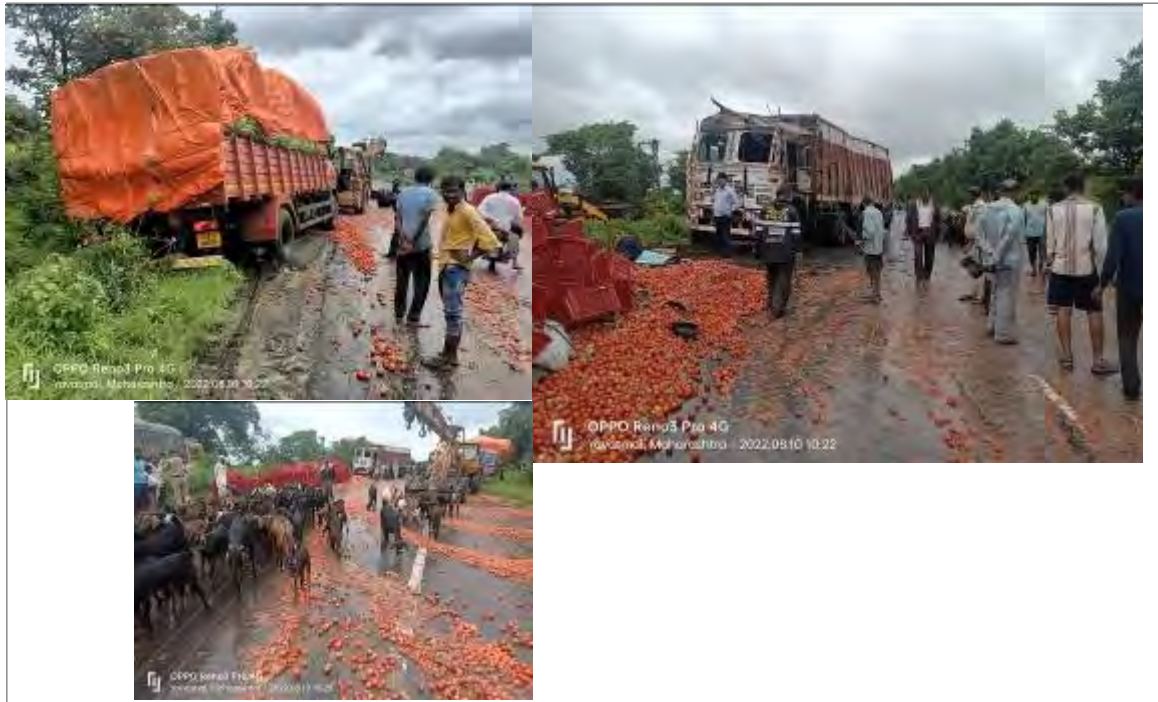
Photo 8: Unbalanced truck accident due to overloading
