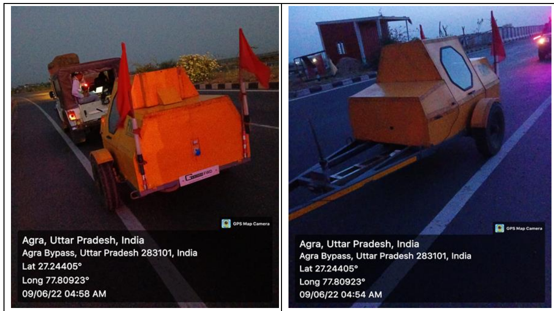
FWD Survey in progress
