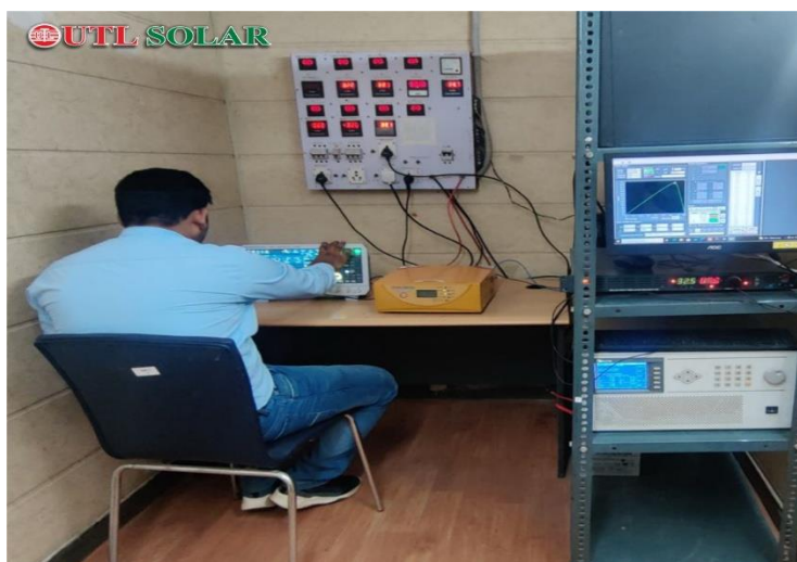
Off grid inverter testing set up
