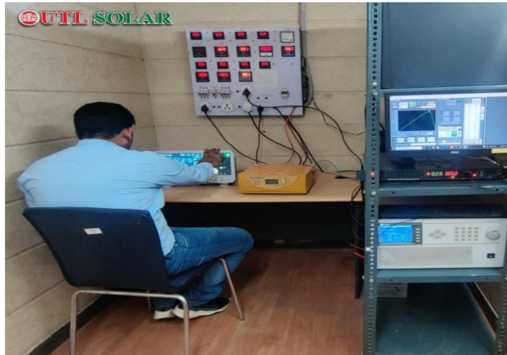
Off grid inverter testing set up
